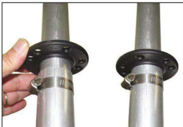
Photo C— Installing the DX Engineering guy rings is easy. Simply slide each one over the appropriate-sized element and let it rest on top of the next larger section. (Photo courtesy of DX Engineering)
