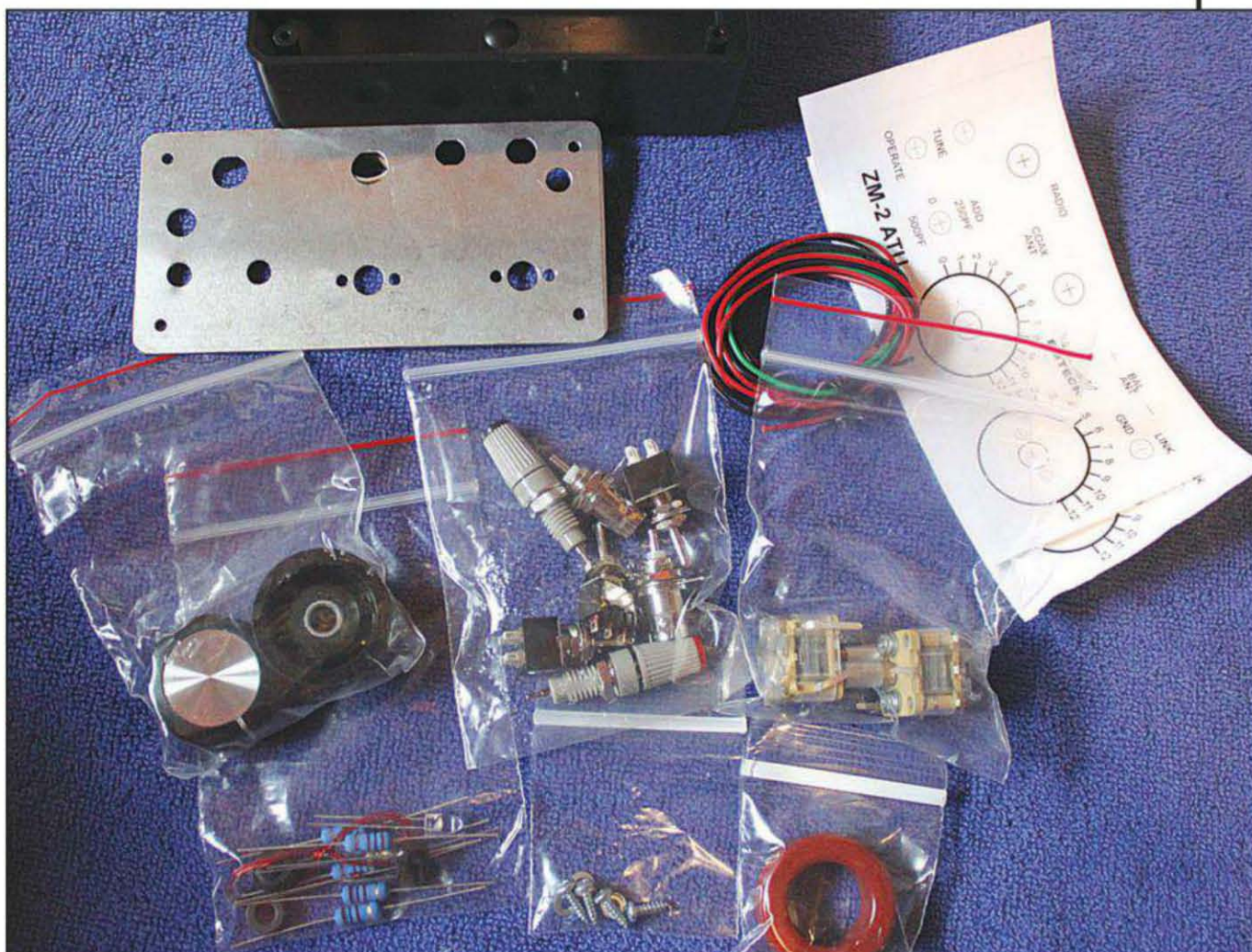
Kit contents as packaged. Notice the large toroid and multiple colors of wires.
