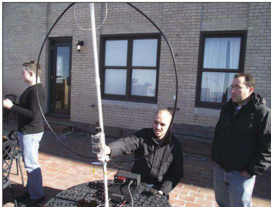
Photo B— The prime operating position at N3Y was a Kenwood TS-50, MFJ travel tuner, and a homemade magnetic loop antenna, provided by Alain De Carolis, WW3WW, center, adjusting the antenna. Watching at the right is Tom Tumino, N2YTF, while Bill Ward, KD4ISF (left), talks with other group members at the second operating position.
