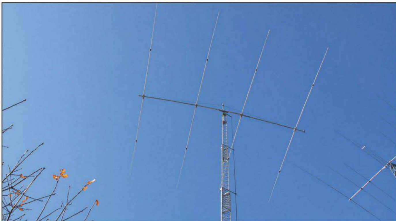
The new 40-meter Yagi where it belongs—high in the air!
