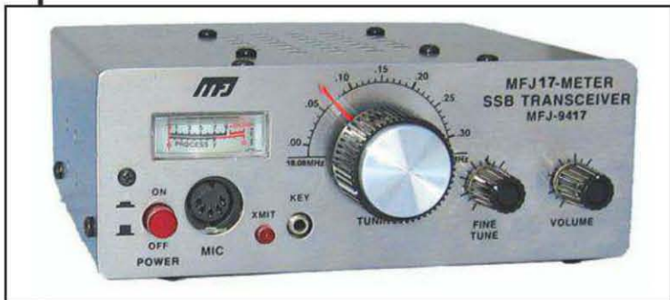
Photo A— The MFJ-9417 is one of two new additions to MFJ's Adventure Radio™ line of portable low-power SSB transceivers. It covers the 17-meter band, while the MFJ-9412 operates on 12 meters. (Photo courtesy MFJ Enterprises)
