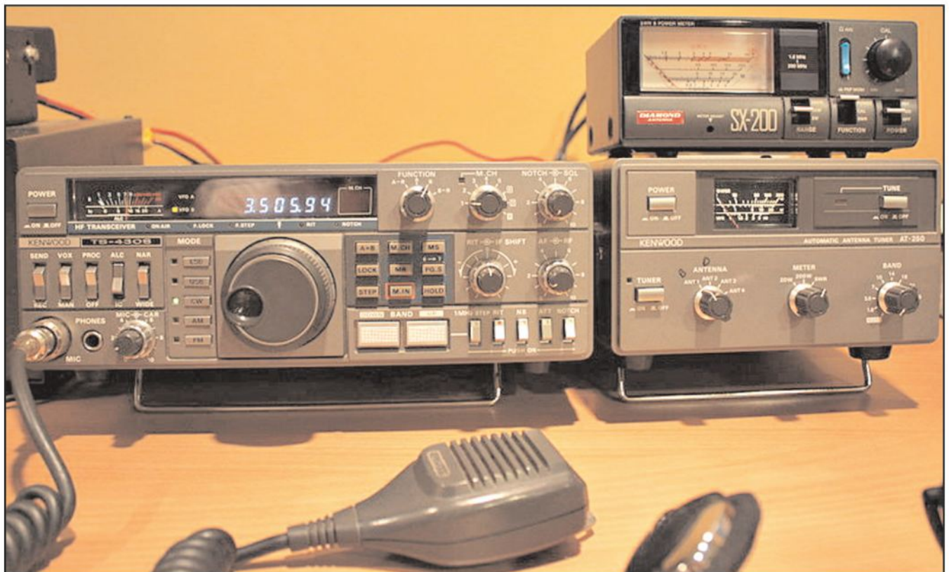
Photo A. With a double Windom antenna, Kurt says there is little to be gained with the use of a remote antenna tuner. This Kenwood TS-430S HF transceiver is paired with the Kenwood AT-250 automatic antenna tuner — which would perform just fine for the questioner's purposes. (Courtesy of ChrisRuvolo via Wikimedia Commons)
