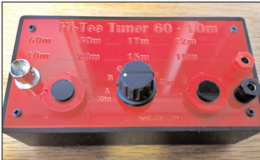
Photo C. The SOTAbears Hi-Tee Antenna Tuner has a front-panel provision for the operator to jot down the dial settings for each band operated. It covers 5 to 28 MHz, the company notes. (Courtesy of SOTAbears)
