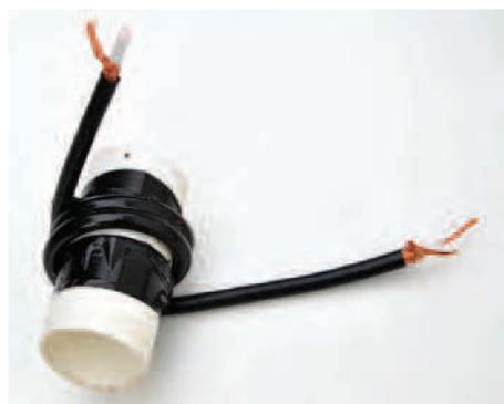
PHOTO 4: A 145MHz current mode choke made simply by winding just over two turns of RG8 Super on a short length of 35mm plastic waste pipe.
