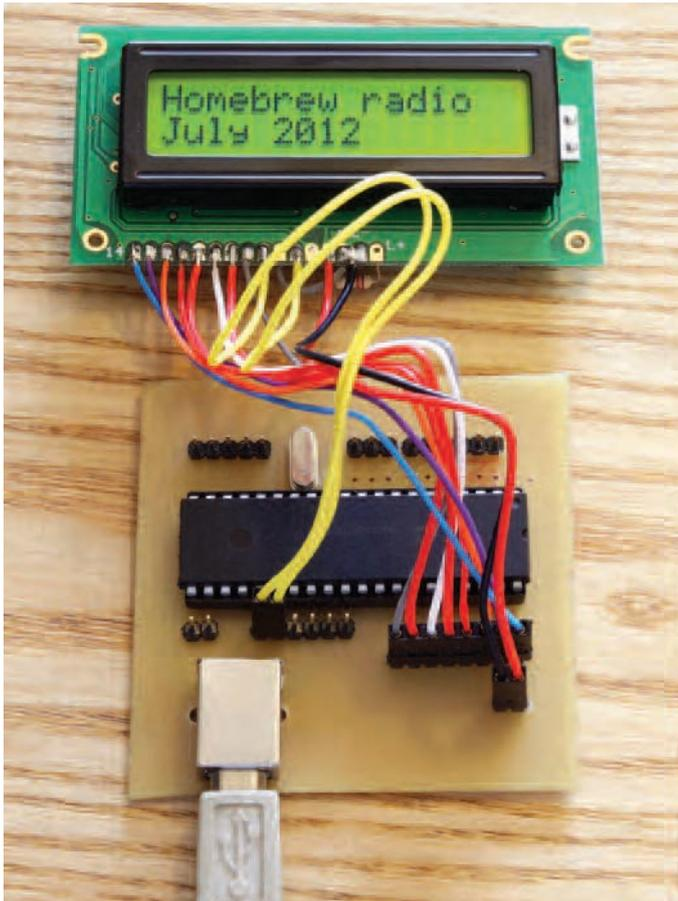
PHOTO 1: My new homebrew Pinguino board driving a LCD display.
