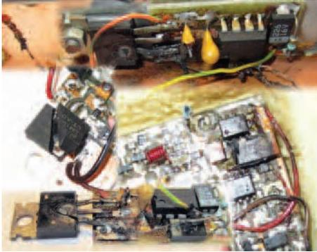
**PHOTO 1:** Montage of typical damage resulting from a sustained overvoltage on the input to regulator chips. These were all the result of a power supply fault triggered by a lightning-induced transient.
