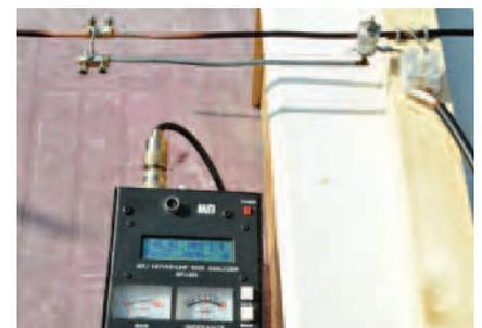
PHOTO 3: Setup for adjusting the antenna gamma match using the MFJ-269.
